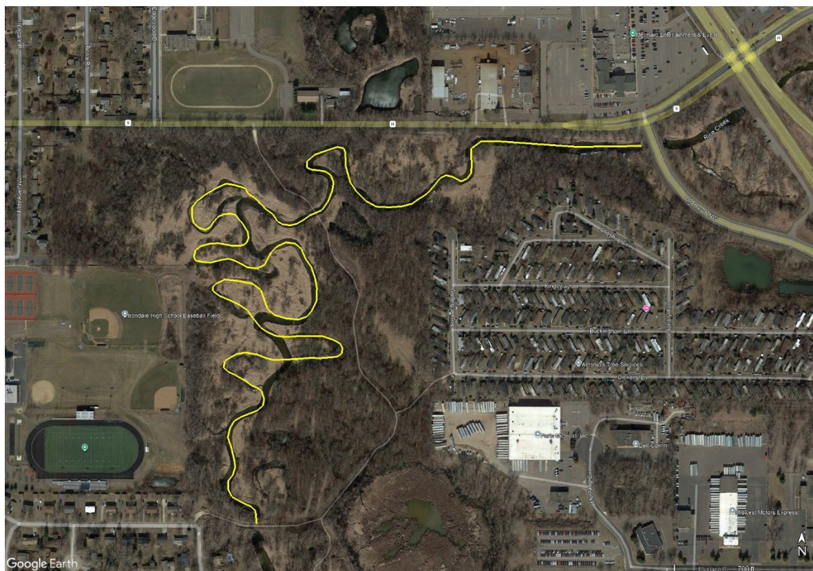
Figure 1. Lower Rice Creek study area. The existing creek length between the two creek crossings is 5,000 LF, and the feasibility study will investigate reconnecting meander cutoffs in the floodplain which could result in an increase of 2,900 LF of creek if implemented (yellow line).
