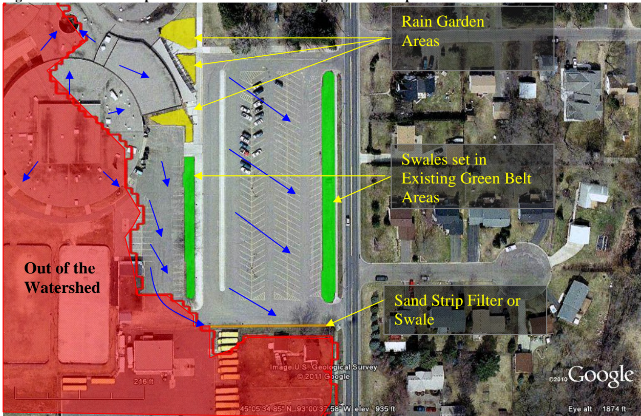
Figure 4.16. Eastern parking lots A and B BMP suggestions. Blue arrows indicate general drainage patterns.
