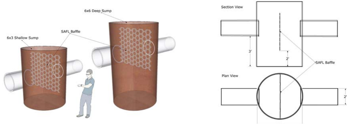
Figure 4.7. The SAFL Baffle is installed in a sump manhole to minimize resuspension of pollutants collected in the sump.
